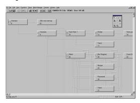
**Graphic or text blocks** gives you flexibility in designing screens for Cimrex model's 30 and up. Text blocks allow you to write multiple text lines easily and printouts are much clearer. Graphic blocks allow you to be creative. Pre-prepared symbols such as tanks, valves, switches, tend graphs, bar graphs, and analog meters are provided, or you can make your own.
