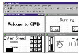
The **3D parts library** is GTWIN's standard library to create touch buttons, bar graphs, message panels, meters, and keypads.
