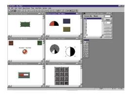
The *3D parts library* is VTSoft's standard library to create touch buttons, bar graphs, message panels, meters, and keypads.
